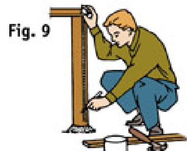
Measure from the top rail to align each bottom rail on each post.
